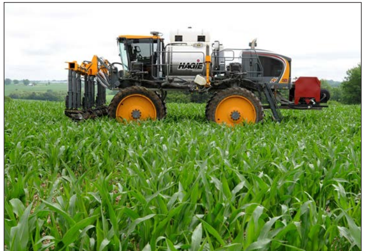
A high-clearance sprayer is used by a northeast Iowa farmer to apply cover crop seed between corn rows.
